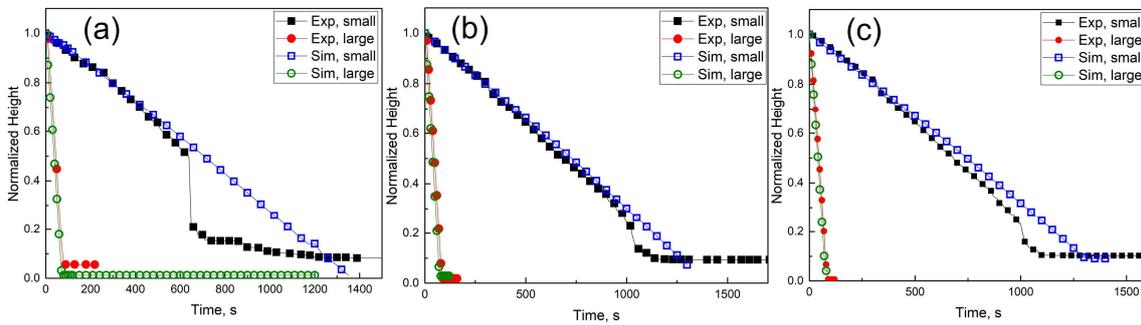
**Fig. S9:** Height vs Time profiles of 100 nm (Upper) and 500 nm (Lower) particles under 4000 rpm, at a mixing ratio = 1:1, comparing the 1-D model to experimental data. Here, (a)  $\phi_0 = 0.01$ , (b)  $\phi_0 = 0.02$ , (c)  $\phi_0 = 0.03$ .
