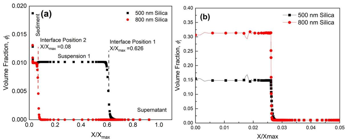
**Fig. S2: (a), simulated concentration profile for a 500:800 nm suspension mixture in 1:1 mixing ratio with  $\phi_0=0.02$  under earth gravity condition after 16 h. The general data are plotted at the spatial points where the solution is calculated according to the meshes.  $X/X_{\text{max}}$  is the relative position. (b) the near-bed zone in detail, which changes to the bidisperse effective maximum volume fraction.**
