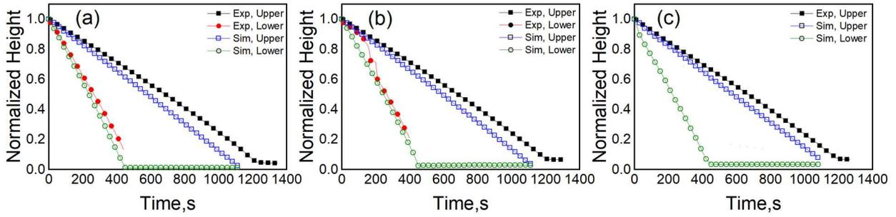
**Fig. S7:** Height vs Time profiles of 500 nm (Upper) and 800 nm (Lower) particles under 1000 rpm, at a mixing ratio = 1:1, comparing the 1-D model to experimental data. Here, (a)  $\phi_0 = 0.01$ , (b)  $\phi_0 = 0.02$ , (c)  $\phi_0 = 0.03$ .
