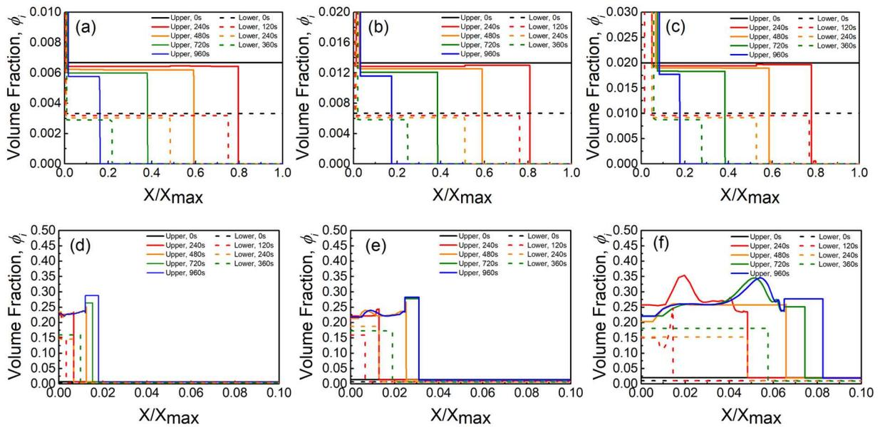
**Fig. S4: Simulated concentration profiles of 500 nm (Upper) and 800 nm (Lower) particles under 1000 rpm, at a mixing ratio = 2:1, using 1-D bidisperse model. (a)  $\phi_0 = 0.01$ , (b)  $\phi_0 = 0.02$ , (c)  $\phi_0 = 0.03$ . (d)–(f), concentration changes in the near-bed region, which changes to the bidisperse effective maximum volume fraction.**
