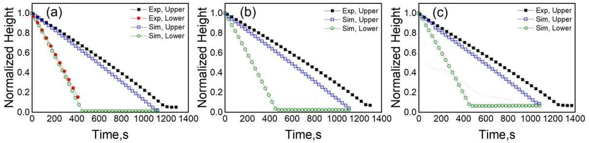
**Fig. S8:** Height vs Time profiles of 500 nm (Upper) and 800 nm (Lower) particles under 1000 rpm, at a mixing ratio = 2:1, comparing the 1-D model to experimental data. Here, (a)  $\phi_0 = 0.01$ , (b)  $\phi_0 = 0.02$ , (c)  $\phi_0 = 0.03$ .
