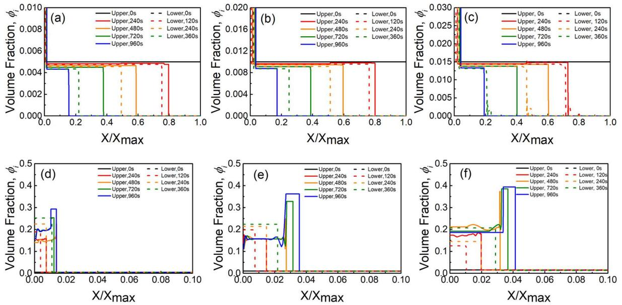
**Fig. S3: (a), simulated concentration profiles of 500 nm (Upper) and 800 nm (Lower) particles under 1000 rpm, at a mixing ratio = 1:1, using 1-D bidisperse model. (a)  $\phi_0 = 0.01$ , (b)  $\phi_0 = 0.02$ , (c)  $\phi_0 = 0.03$ . (d)–(f), concentration changes in the near-bed region, which changes to the bidisperse effective maximum volume fraction.**
