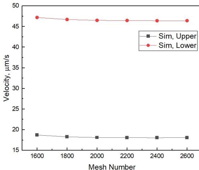
**Fig. S1: Independence grid verification using 500 nm (Upper):800 nm (Lower) particles under 1000 rpm and a mixing ratio = 1:1.**
