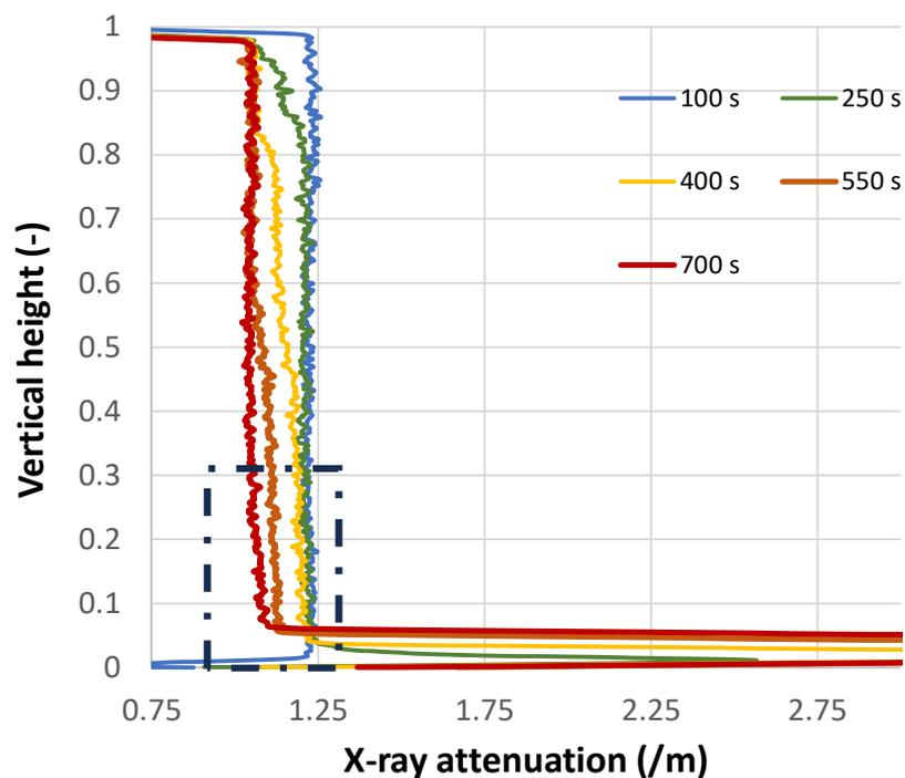
**Fig. S5:** Normalized X-ray sedimentation data, presenting total attenuation versus sample height for a 500:800 nm suspension at a mixing ratio 1:1 and total volume fraction,  $\phi_0 = 0.03$ . Full profile shown in the figure and expanded near-bed zone shown in Fig. 4 is the dashed box.
