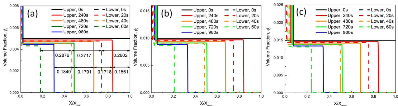
**Fig. S6:** Simulated concentration profiles of 100 nm (Upper) and 500 nm (Lower) particles under 4000 rpm and a mixing ratio = 1:1. Here, (a)  $\phi_0 = 0.01$ , (b)  $\phi_0 = 0.02$ , (c)  $\phi_0 = 0.03$ .
